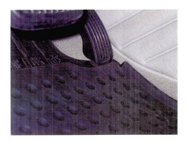
Note: AWM cannot interfere with accelerator pedal if properly secured with the retention clips
